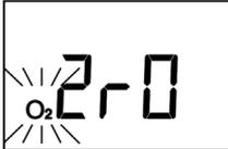
3. **Calibration is successfully completed** when the detector displays the gas concentration with sequential activation of the buzzer, vibration and flashing of the LEDs.
