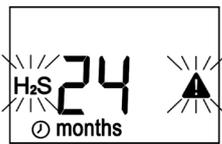
If **be safe SG** fails the self-test, the warning icon “▲” will appear flashing and the icon of the type of the sensor will start flashing. **be safe SG** will then have to repeat the self-test.
