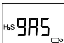
4. From the inspection screen, expose the instrument to the relevant gas for 45 seconds.
