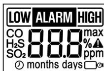
3. Then, the display shows the low alarm (LOW ALARM) and high alarm (HIGH ALARM) settings. These data can be set using the PC software '**Be Safe SG IR-Link manager**' (see Appendix A):
