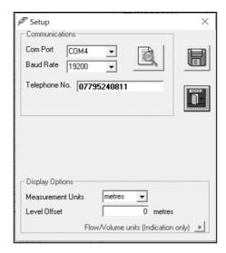
UltraLog will set up the comms port you will be using to the following configuration.
