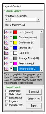
The Legend Control is used to edit and modify the data displayed in the current chart and can be toggled On and Off by pressing the top icon of the line of icons which run down the left-hand side of the Chart window.
