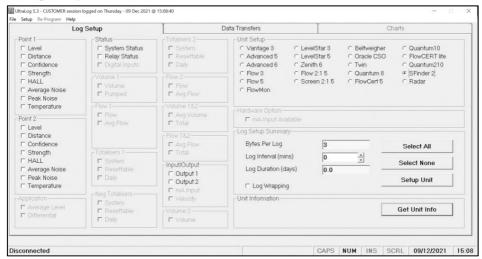
The Log Setup screen is used to program the Pulsar Ultra series, fitted with an optional Data Logging board to log the required data.
