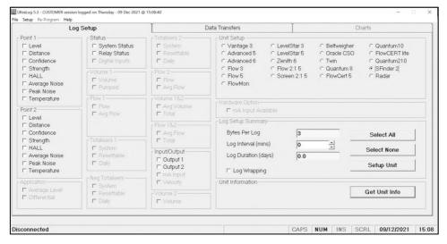
The screen shown above would appear if a SludgeFinder2 was selected. The ticked circle in the 'Unit Setup' window at the top right hand of the display indicates the unit type, which is verified after the 'Get unit Info' button is pressed, and the unit is interrogated. Any 'greyed out' option is not able to be logged with the system type selected.
