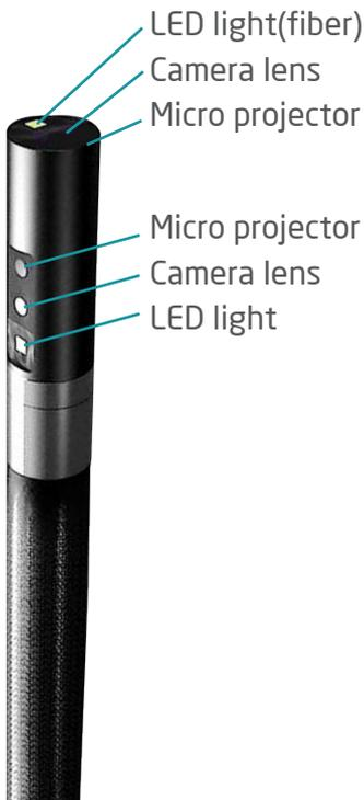
The tip end contains two pairs of Micro projector/Camera lens/LED light on the front view (0°) and the side view (90°) directions.
