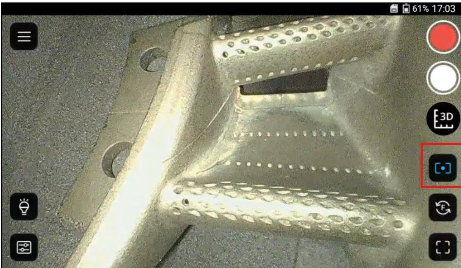
The system default auto exposure point at center. User can tap any position on screen live view to focus the exposure value, then the focus button on the right side will turns on. Tap the button again to back to default setting.
