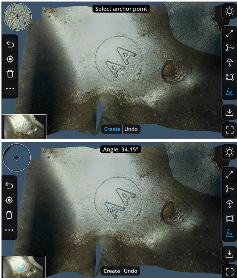
1. Set the anchor point and two end points to measure the angle.
