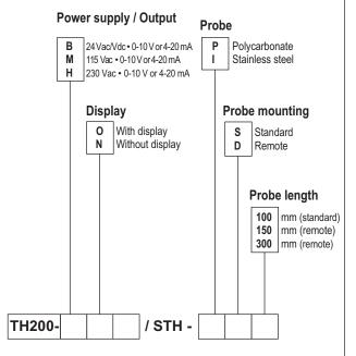
**Example : TH200-BN/STH-PD300** = humidity transmitter type TH200, with 24Vac/Vdc power supply, without display with polycarbonate remote probe length 300mm
