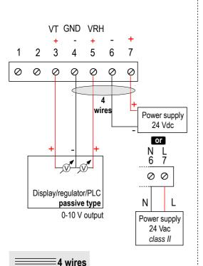
To make a 3-wire connection, before powering up the transmitter, please connect the output ground to the input ground. See drawing below.
