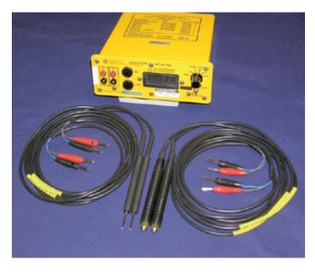
In areas where there is flammable gas present the 1681B does not present a hazard since it is certified for use in an ATEX zone I environment. The rugged aluminium case has very low magnesium content and is proof against a number of liquid contaminants such as Aviation fuel, De icing fluid and Methanol.
